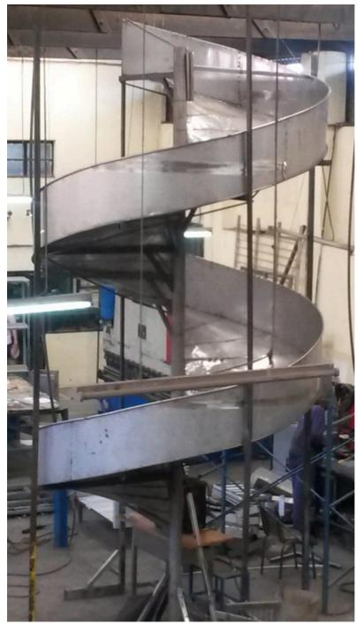
The Stainless Steel Spiral Bread Chute is designed for the smooth, controlled descent of bread products from elevated conveyors to lower levels, minimizing impact and preserving product integrity. Fabricated from high-grade stainless steel, it ensures durability, hygiene, and compliance with food industry standards. **Key Features:**
