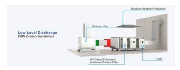
Stainless Steel Products Limited **Description**: An air purifier is a powerful solution for improving air quality in commercial kitchens by removing pollutants, odors, and chemicals. Activated charcoal effectively traps contaminants such as volatile organic compounds (VOCs), smoke, cooking smells, and grease, making it ideal for high-traffic cooking environments where air quality can quickly degrade.
