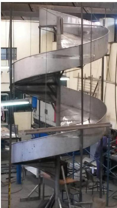
The Stainless Steel Spiral Bread Chute is designed for the smooth, controlled descent of bread products from elevated conveyors to lower levels, minimizing impact and preserving product integrity. Fabricated from high-grade stainless steel, it ensures durability, hygiene, and compliance with food industry standards. Key Features:
